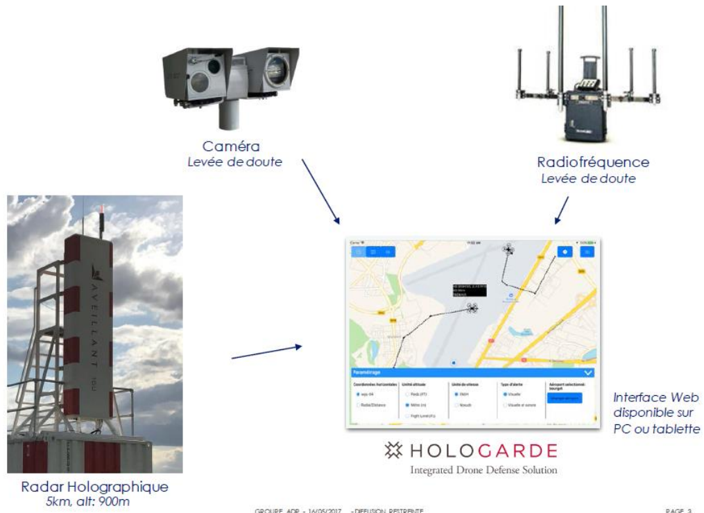
Figure 3: The HOLOGARDE system, able to detect a small drone 5 km away
